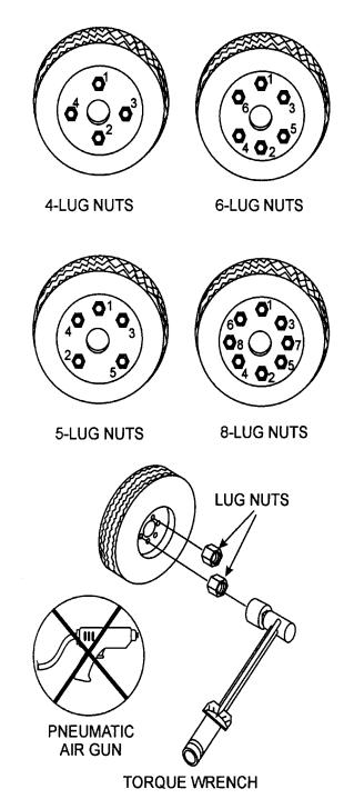
Figure 3. Wheel Lug Nuts Tightening Sequence
